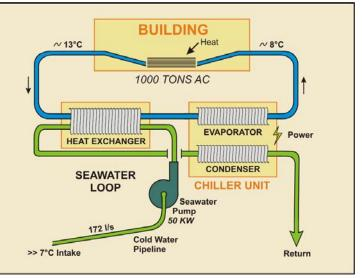
exposure. This is illustrated below. The fresh chill water is first cooled by seawater through a heat exchanger and then secondarily cooled with an auxiliary chiller. The auxiliary chiller is basically a refrigeration system with its condenser cooled by the returning flow of cool seawater. With the condenser kept cool, the auxiliary chiller can operate at an extremely high efficiency – as high as double that of a conventional chiller.
