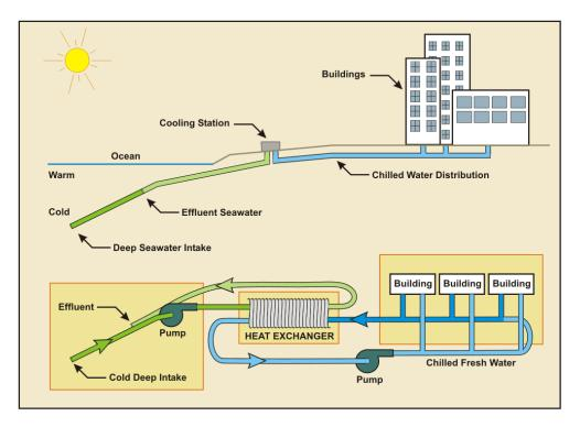
The main components of a seawater air conditioning system are the seawater supply system, the heat exchanger or cooling station and the fresh water distribution system. These basic components can be optimized for each specific location, climate and building.
