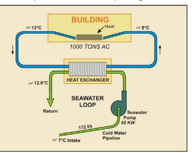
offshore and have a nominal intake depth of 700 m. The effluent seawater is discharged though a second pipe at a depth of approximately 40 m.
