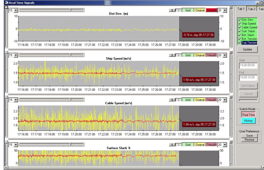
MakaiLay provides graphical output showing actual and desired cable payout rates and distances.
