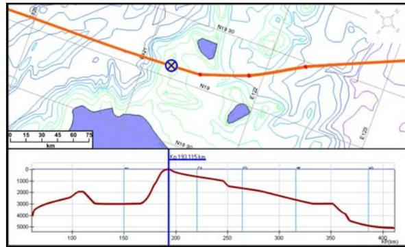
**Figure 1.** Cable route planners can now link plan and profile views to efficiently manage the cable route design process. Routes are edited using click and drag techniques and precise RPL and cable assembly lists and diagrams are created automatically.
