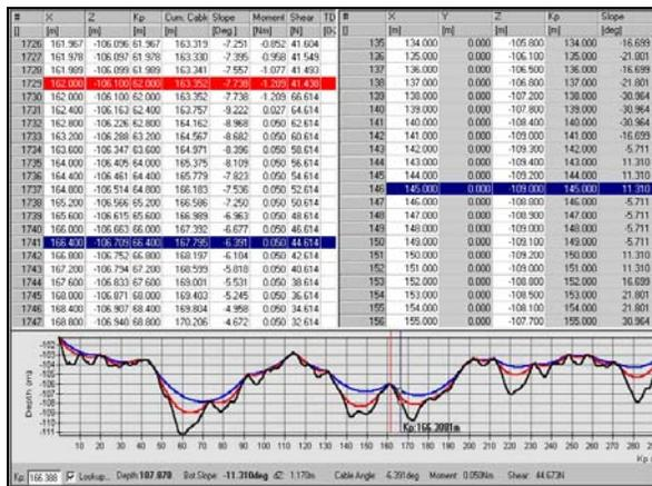
**Figure 4.** Example of cable suspension analysis for two different tensions.
