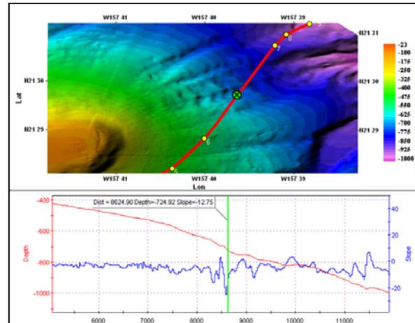
**Figure 3.** User can interactively create and modify the routes and reference lines, and depth profiles and slope graphs are automatically generated.
