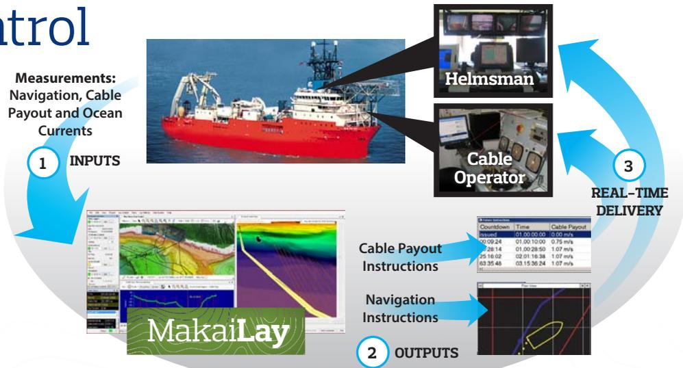
**The Control Loop:** MakaiLay logs and processes data from the ship's instruments. The 3D Cable model then computes the cable payout and navigation instructions to maintain the desired bottom conditions. MakaiLay then issues these instructions to the helmsman and the cable operator in real-time.
