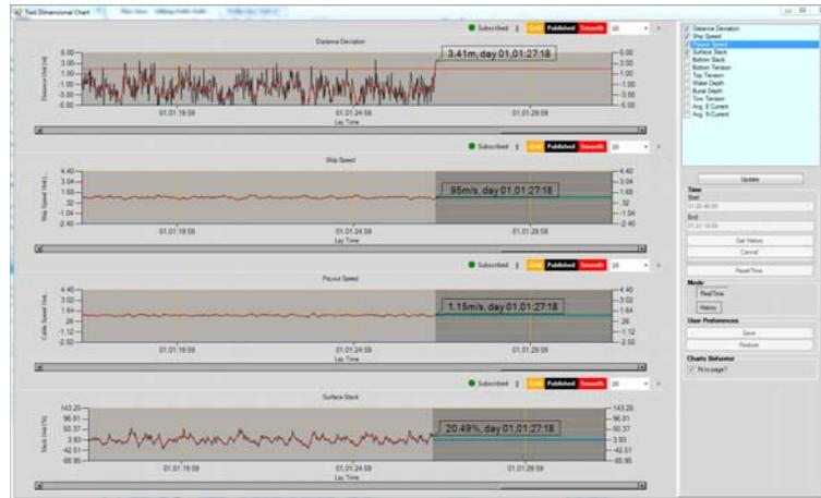
*MakaiLay provides real-time charts showing the actual vessel and cable engine measurements, as well as the desired navigation and cable engine instructions.*
